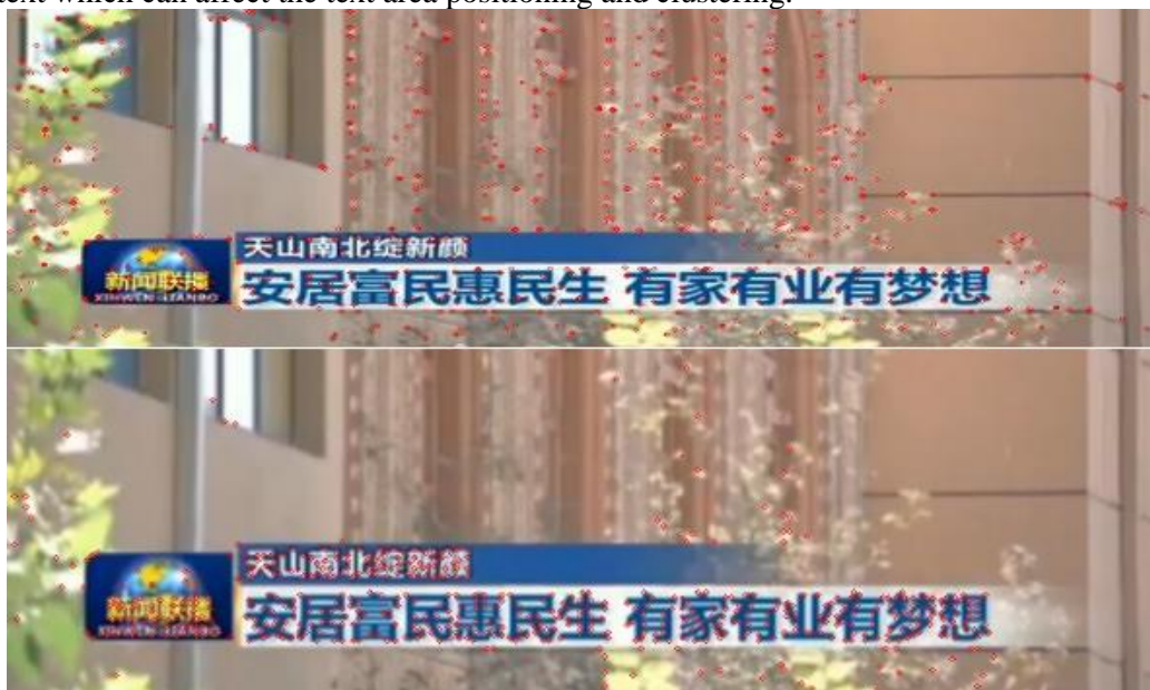
Figure 5. Compared Results between Harris Algorithm and the Method Used in This Project of Corner Detection
