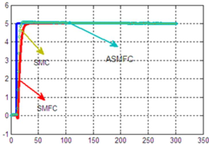
**Figure 5. Third link trajectory without disturbance**
