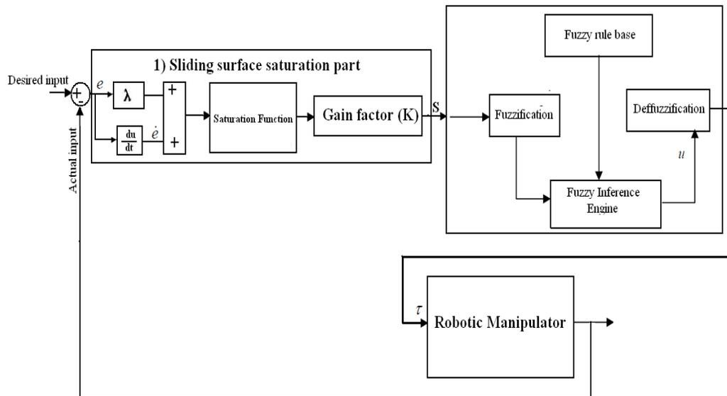
**Figure 2. Sliding Mode Fuzzy Control of robot manipulator (SMFC).**
