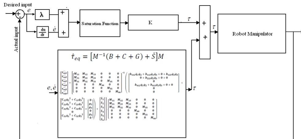
Figure 1 Block diagram of classical sliding mode controller
