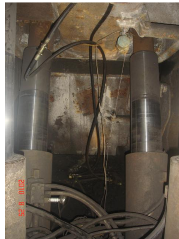
Figure 4c. Leg closure recorder fitted in the legs
