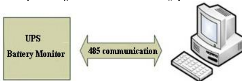
Figure 2. The Design of Local Real-Time Monitoring System
