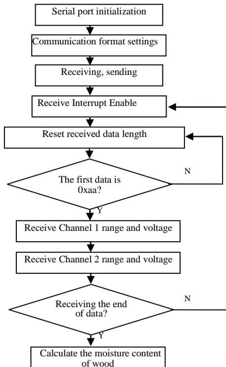
**Figure 6. Main Controller Collection Procedures with Wood Moisture Communication Flowchart**
