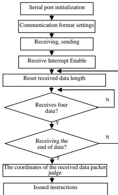
**Figure 5. Touch Screen and Master Communication Flowchart**
