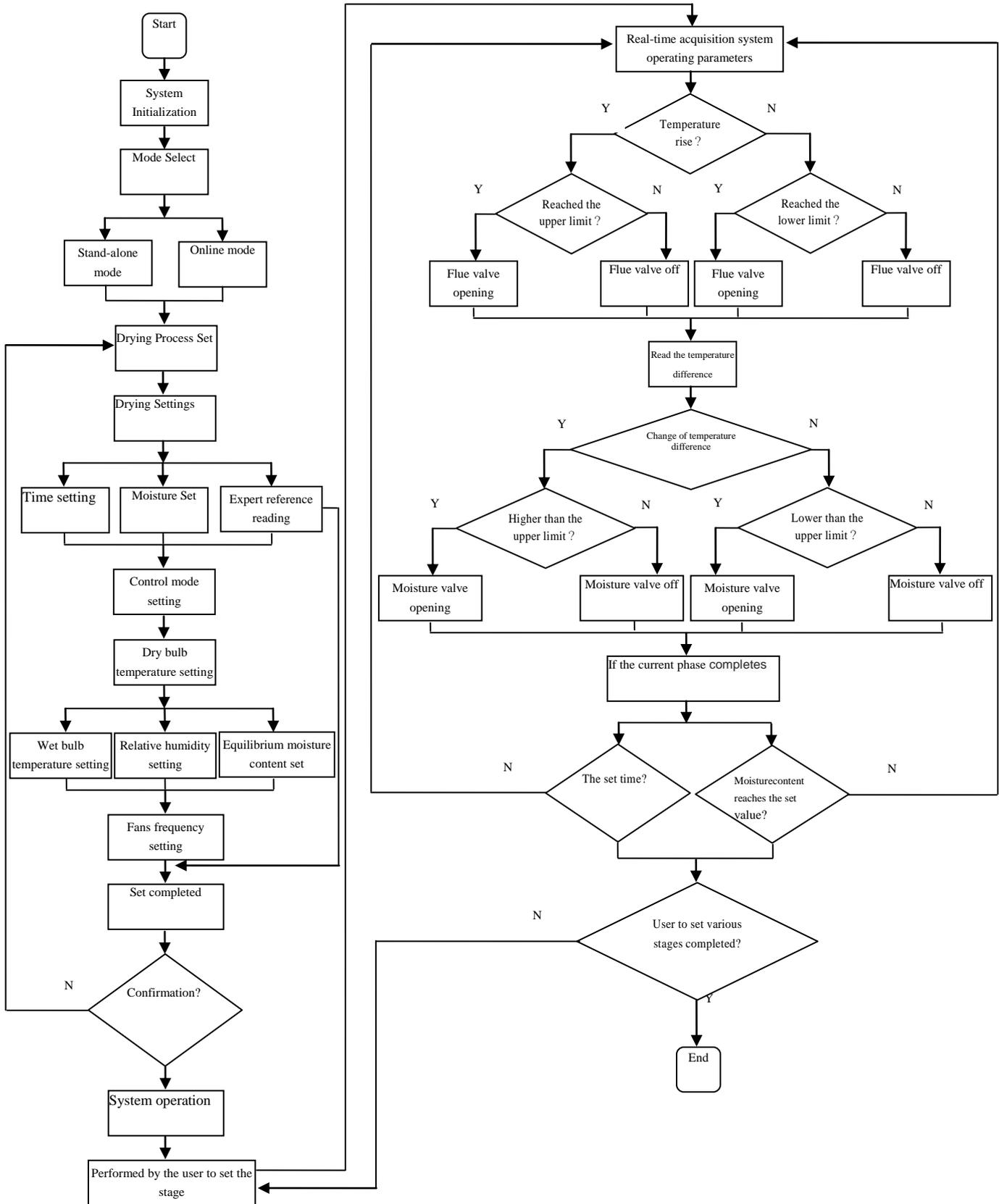
Figure 4. System Control Program Flow Chart
