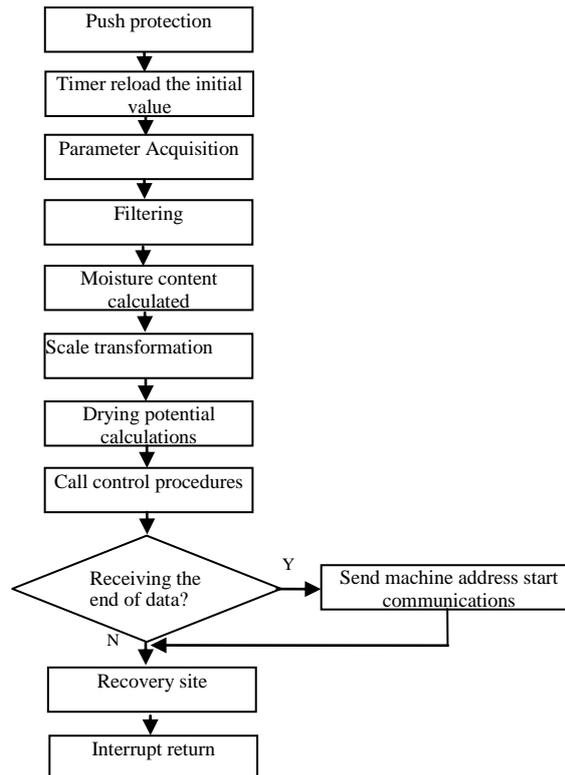
**Figure 7. Drying Kiln Parameter Sampling Interrupt Program Flow Chart**
