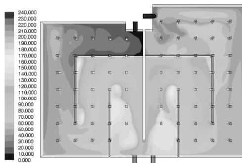
**Figure 9. Solid Figure of Residence Time Distribution in Clearwell Reaching 1.0 m Under Average Influx**
