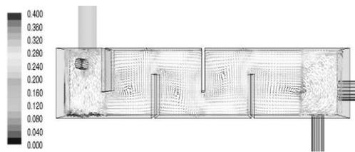
**Figure 3. Plane Figure of Vector in Clearwell Influx**
