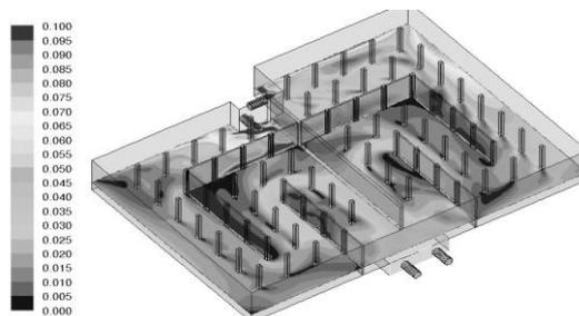
**Figure 6. Solid Figure of Vector in Clearwell Reaching 1.0 m Under Average Influx**
