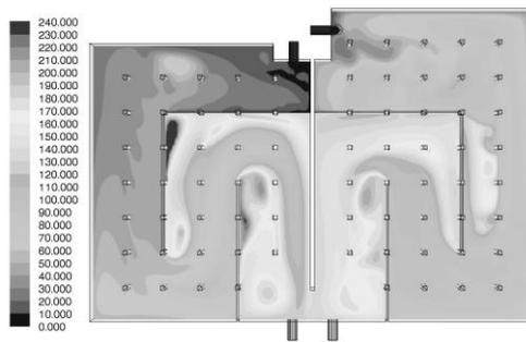
**Figure 11. Solid Figure of Residence Time Distribution in Clearwell Reaching 1.0 m Under Minimum Influx**
