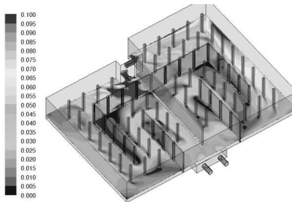
**Figure 8. Solid Figure of Vector in Clearwell Reaching 1.0 m Under Maximum Influx**
