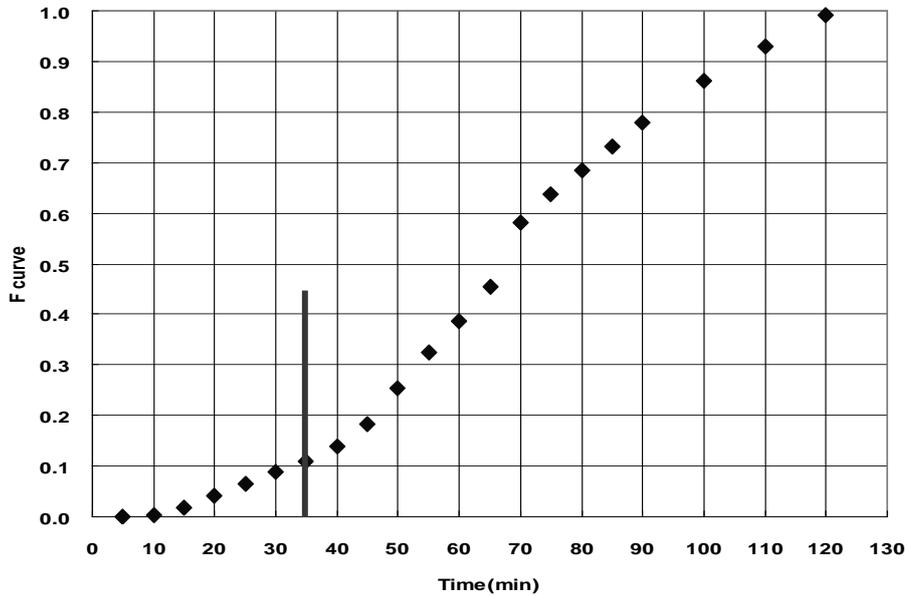
**Figure 12. T<sub>10</sub> of F Curve as Tracer Test**
