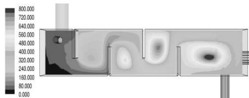
**Figure 4. Plane Figure of Residence Time Distribution in Clearwell Influx**
