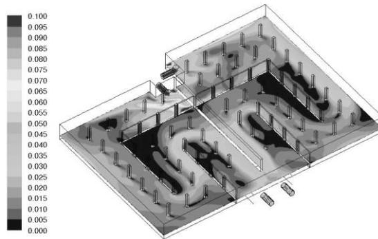
**Figure 7. Solid Figure of Vector in Clearwell Reaching 1.0 m Under Minimum Influx**
