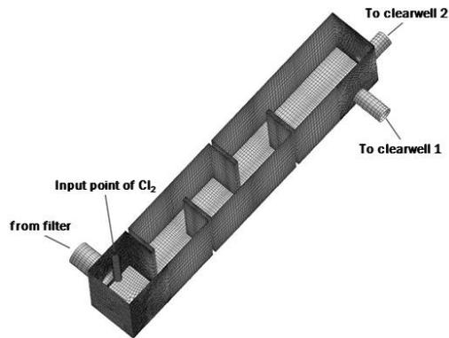
**Figure 2. Model of Influx in Clearwell**
