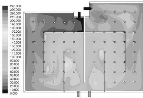
**Figure 10. Solid Figure of Residence Time Distribution in Clearwell Reaching 1.0 m Under Maximum Influx**
