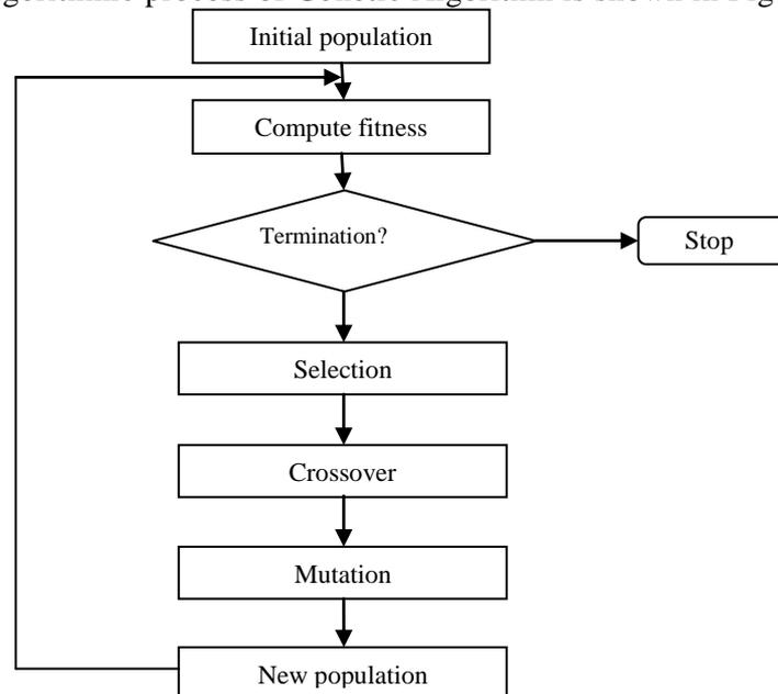
Figure 1. The Algorithmic Process of GA
