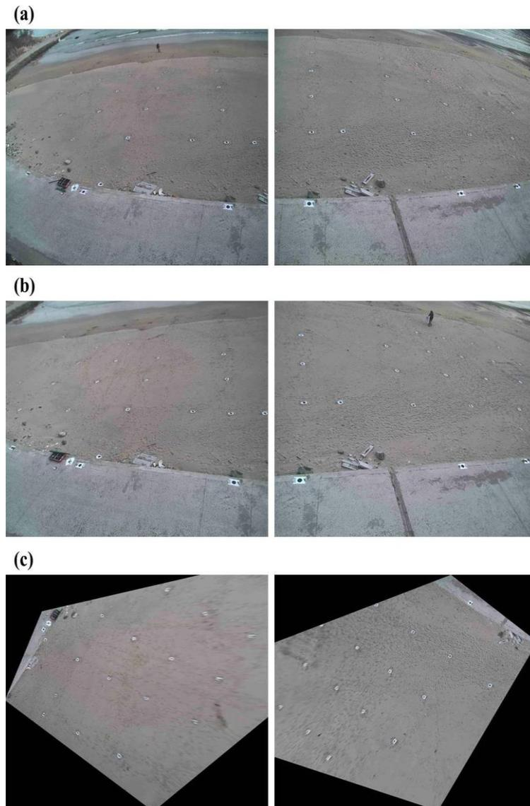
**Figure 4. The Geometric Distortion Correction for a Network Camera: (a) Original Photographic Image from the GCPs for Camera 1 and Camera 2 Installed on the Beach, (b) Image Corrected for the Distortion of the Camera Lens, and (c) Geometric Correction Results for Distortion-Corrected Images**
