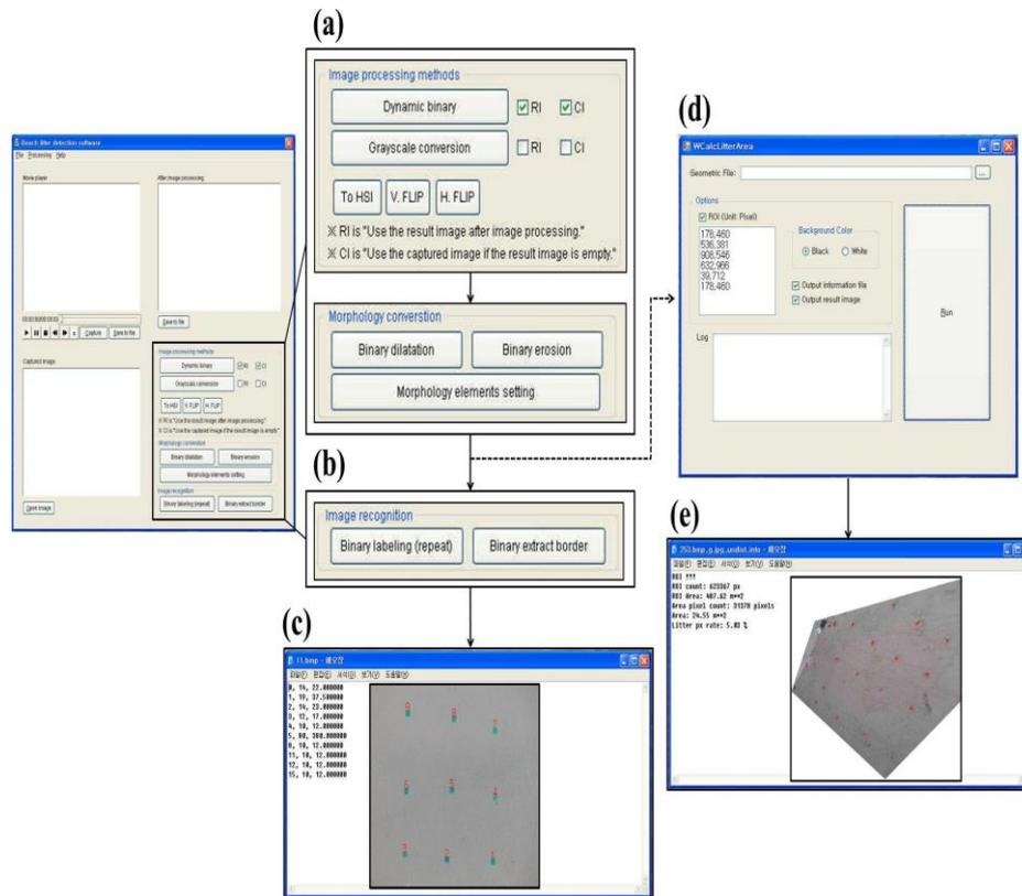
**Figure 5. The Structure of the Beach Litter Detection (BLD) Software: (a) Image Pre-Processing and the Morphology Function for Noise and Background Elimination from the Remotely Monitored Image, (b) and (c) Image Recognition Function for the Calculation of Beach Litter and a Background-Eliminated Unmanned Aerial Vehicle Image, and (d) and (e) Result of using the BLD Software to Calculate the Area of Beach Litter from Background-Eliminated Networked Camera Images**
