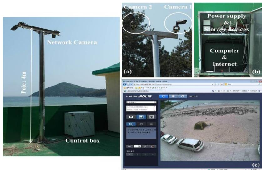
**Figure 2. The Structure of the Network Camera System: (a) a Network Camera Setting on a 4-m-high Pole (SNO-7080R), (b) the Structure of the Control Box, and (c) the Web Browser for Real-Time Monitoring**
