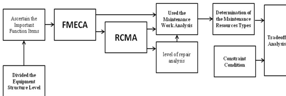
**Figure 2. General Process of Maintenance Support Resources Demand Analysis**
