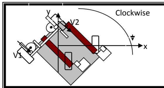
Figure 8. Rotation Corresponding to "RIGHT" Voice Command
