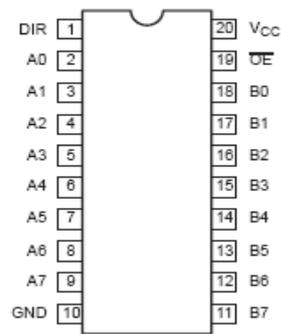
**Figure 5. Pin Configuration of 74ABT245**
