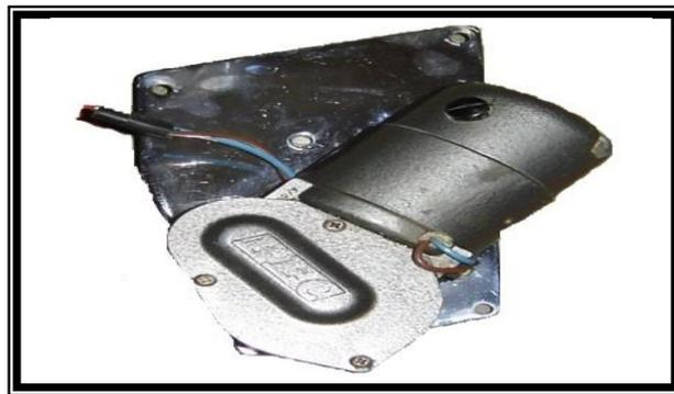
Figure 2. DC Motor Used In Wheelchair
