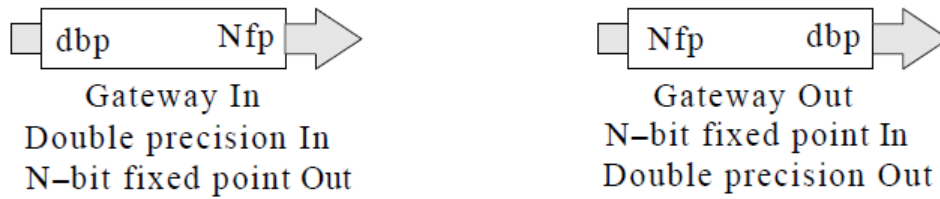
Figure 6. Symbols for Conversion from Double to N-bit Fixed Point and Vice Versa
