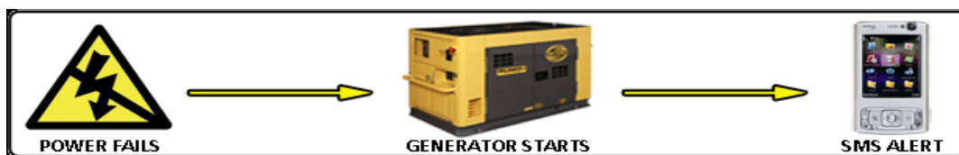
Figure 1. GSM based Power Failure Indicator
