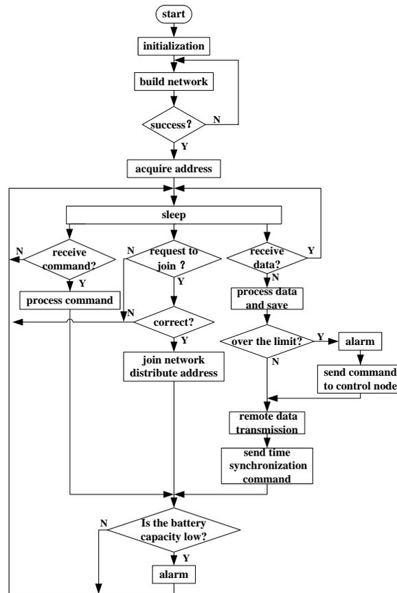
**Figure 8. Software Flow Diagram of the Coordinator Node**
