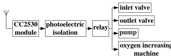
**Figure 5. Circuit Block Diagram of the Control Node**
