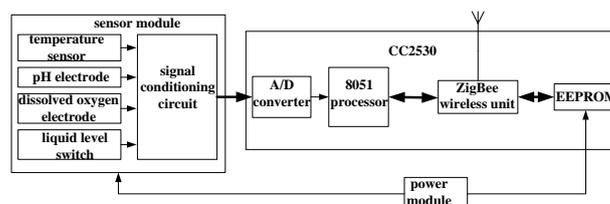
Figure 2. Circuit Block Diagram of the Sensor
