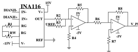
**Figure 4. Signal Conditioning Circuit of the pH Electrode**
