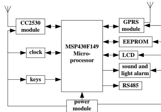
**Figure 6. Circuit Block Diagram of the Coordinator Node**
