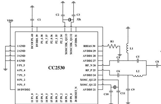
**Figure 3. Peripheral Circuits of the CC2530**
