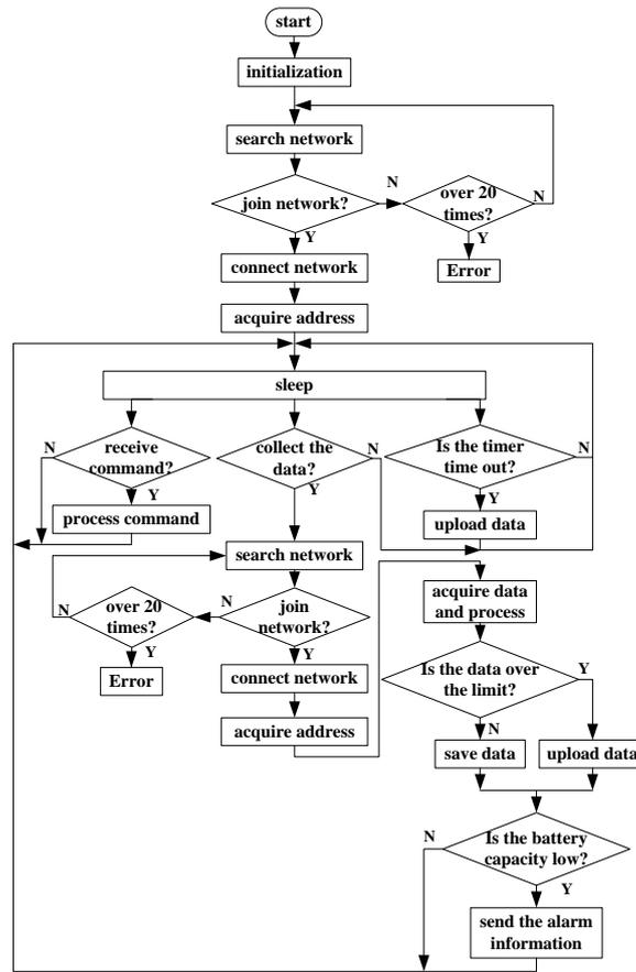
Figure 7. Software Flow Diagram of the Sensor Node
