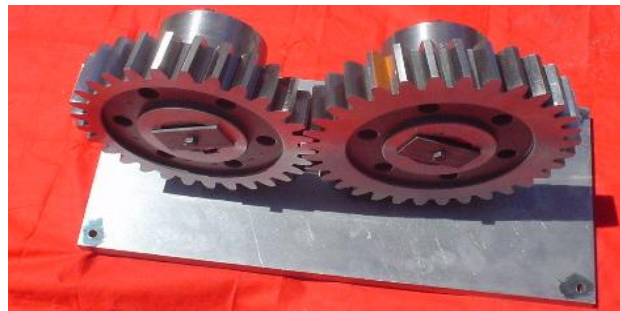
Figure 5. Cross-axis Thickening of Non-involute Gear
