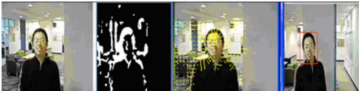
Figure 6. Object Tracking based on Optical Flow
