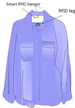
Figure 4. Location of RFID tag and Smart RFID hanger
