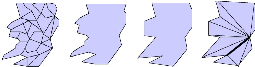
(a)Original mesh (b)Superface creation (c)Border straightening (d)Superface triangulation
