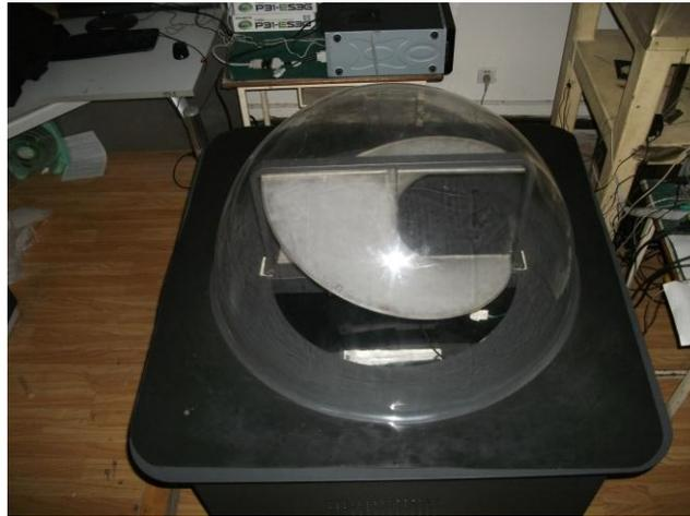
**Figure 1. The Third Prototype of the Volumetric-swept Display System**
