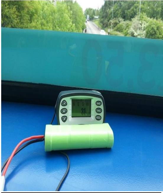
Figure 1. PerformanceBox Mounted on the Top Deck Dashboard of the Double Decker Bus
