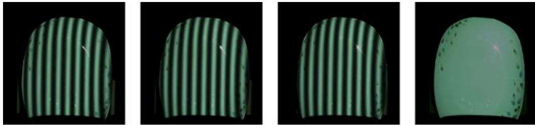
Figure 8. The Diagram of Projected Sinusoidal Phase Shift Code
