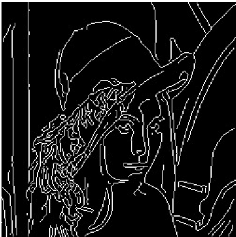
Figure 1.(c) Result of Canny Detection
