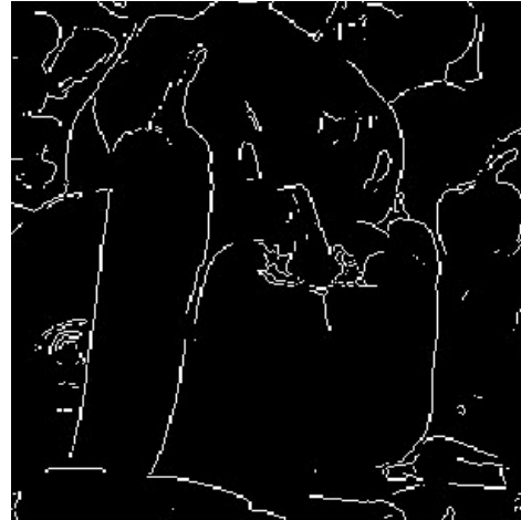
Figure 2. (b) Result of Sobel Detection
