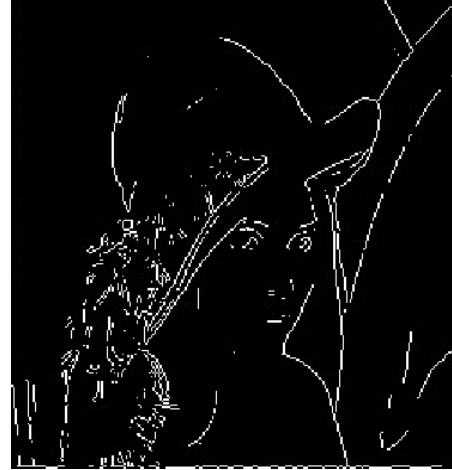
Figure 1. (b) Result of Sobel Detection
