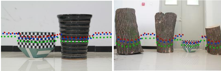
Figure 7. Projection of the Laser Points into the Images with the New Method (Green), the Method in Zhang (Red) and the Method in Li (Blue)
