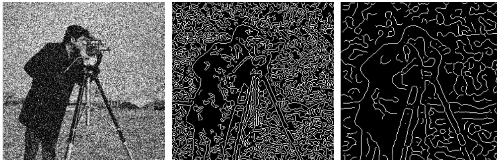
(d) Original Image with Noise (e) Canny Operator (f) The improved Operator
