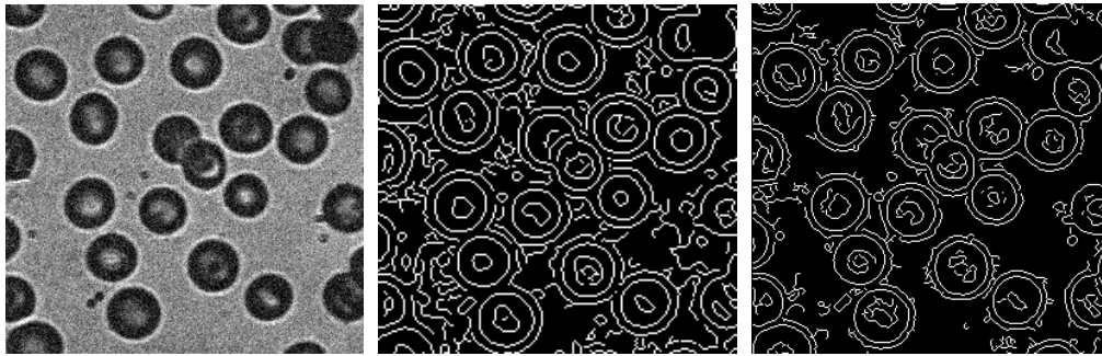
(d) Original Image with Noise (e) Canny Operator (f) The improved Operator
