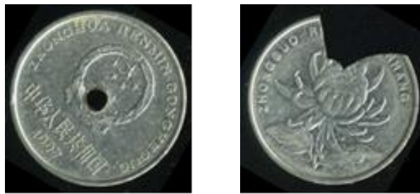
(a)Incomplete of 1yuan (b) Incomplete of 1jiao
