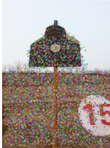
Figure 3. SIFT Feature Points Extracted from Target Image
