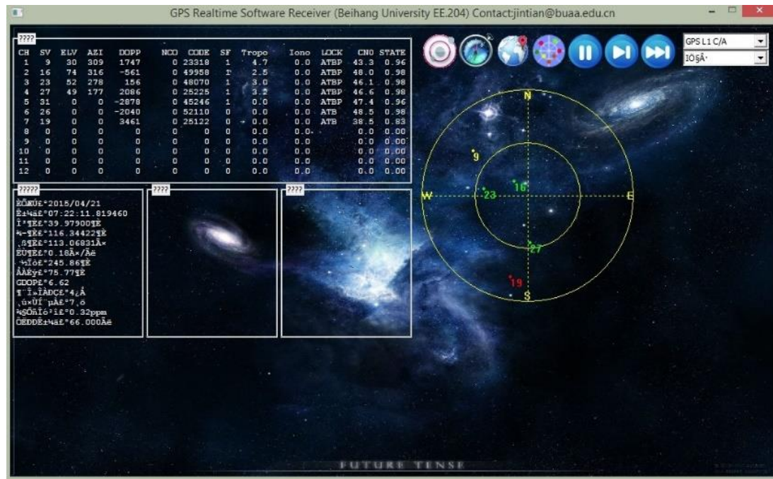
Figure 13. Result of GPS Positioning with Display the Visible Satellites
