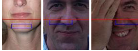
Figure 16. Incorrect Results of Lips Detection Algorithm
