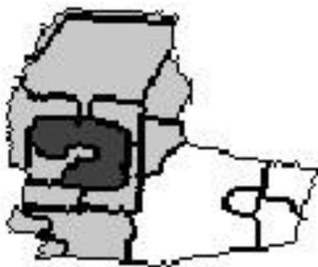
Figure 4. Search Start Point and Shadow Candidate Area of Vehicle Body
