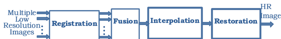
Figure 1. The Generalized Block Diagram of Super Resolution
