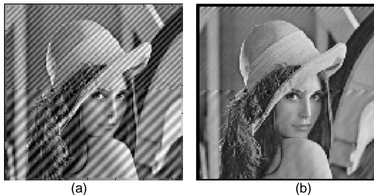
Figure 6. Restoring when the Sinusoidal Disturbance Added to the Image is of a Varying Frequency: (a) The Image with the Disturbance (b) The Restored Image
