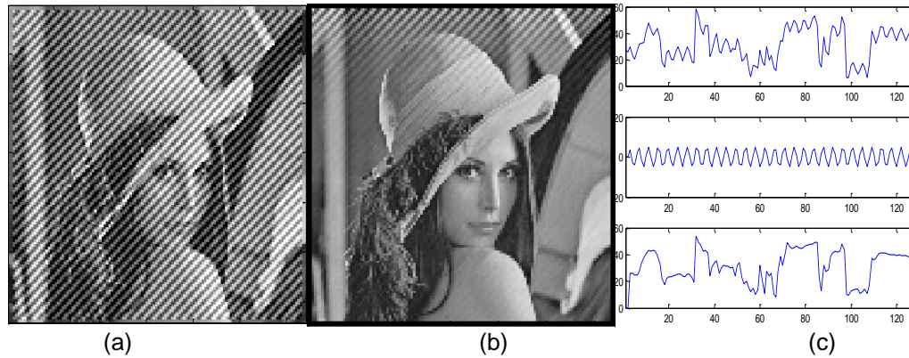
Figure 5. Restoring when the Sinusoidal Disturbance Added to the Image is a Shifted and Scaled Version of the Reference Sinusoidal Input (a) The Image with the Disturbance (b) the Restored Image (c) One Line from Input Image (Top), the Reference Sinusoidal Image (Middle) and the Restored Image (Bottom) with the Disturbance Removed
