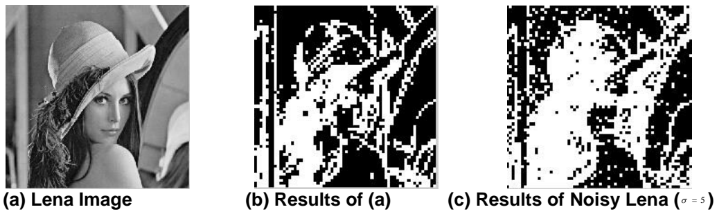
Figure 4. Classification Results from DCT Method: the Black and White Indicate Smooth and Non-smooth Patches Respectively
