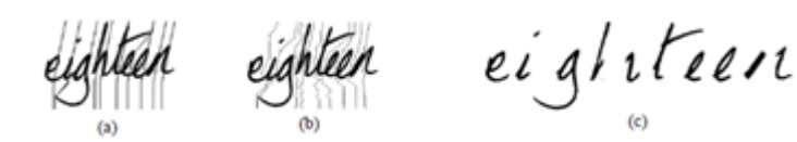
Figure 2. Segmentation using Shortest Path of a Graph of Gray Level Image (a) Segmentation Intervals (b) Segmentation Paths (c) Segments [11]
