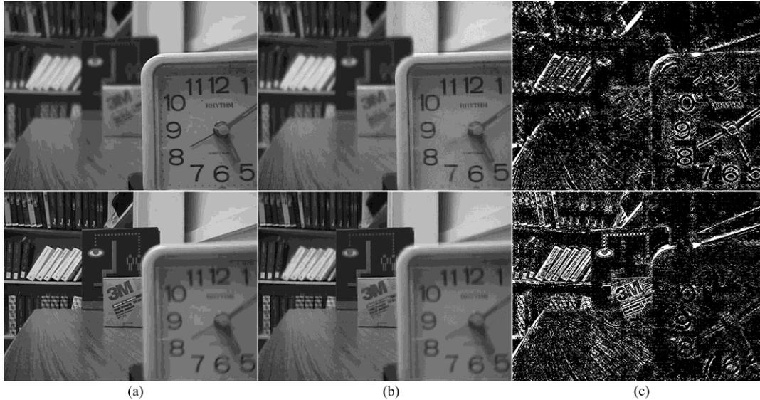
**Figure 2. Decomposition of Multi-Focus Images 'Disk' using RPCA (a) source Images, (b) Principal Components, (c) Sparse Components**
