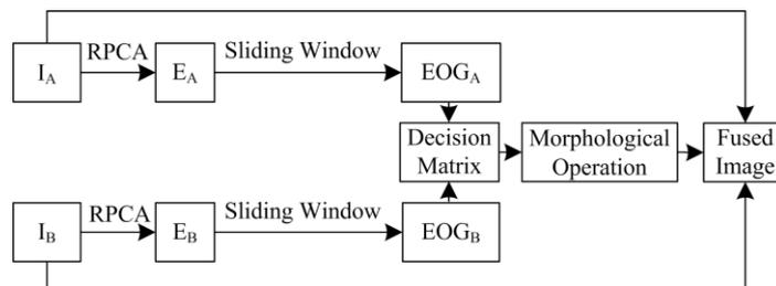
**Figure 1. Block Diagram of Proposed Multi-Focus Images Fusion Framework**
