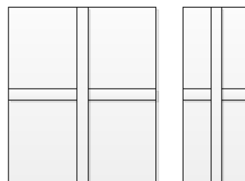
Figure 4. Geometry of Concentrically Stiffened Isotropic Plate with Two Orthogonal Stiffeners
