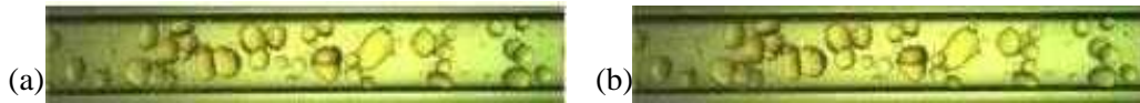
Figure 3. Original Images of Oil-Water Two-Phase flow in Horizontal Pipe with 5\text{m}^3/\text{d} -80% Condition; (a) The 853th Frame Original Image; (b) The 854th Frame Original Image
