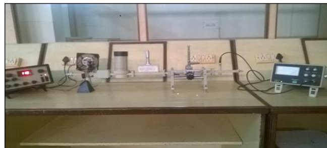
Figure 4. Microwave Bench Setup for the Measurement of Microwave Absorption
