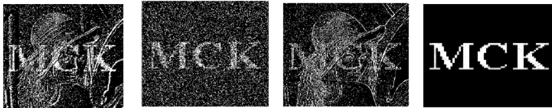
Figure 4: a) Resizing; b) Gaussian Noise (512,256,512) (mean=0, variance 0.001); c) High Pass Filter [0.6]; d) JPEG Compression
