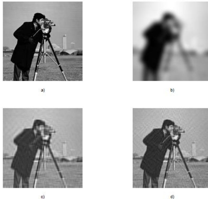
Figure 2. a. Original image of 256 × 256 pixels b. Blurred image with Gaussian distribution, mean 0, variance 8 and reflexive boundary conditions c. Image restored by the Barzilai-Borwein algorithm after 2408 iterations d. Image restored by the conjugate gradient algorithm after 4089 iteration
