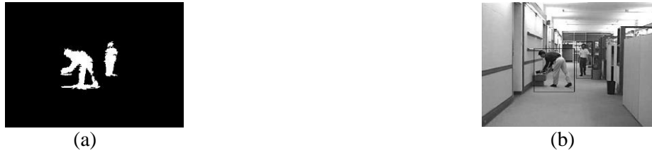
Figure 6. (a) Image showing object's maximum displacement within 8 frames; (b) Creation of rectangular bounding boxes covering the region of maximum displacement by the object
