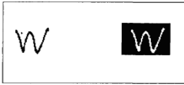
Figure 2.3. Effect Diagram of Median Filtering
