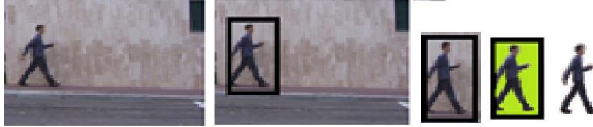
Figure 6. (a) Incoming Frame (b) Interest Point Detection (c) Region of Interest (d) Computations on Region of Interest (e) Extracted Silhouette
