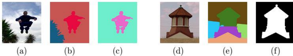
Figure 4. Comparisons of the segmentation results by graph segmentation[15] based on grid graph and nearest neighbor graph. Panels (a),(d) are the original images. Panels (b),(e) show the segmentation results by graph segmentation based on grid graph. Panels (c),(f) show the segmentation results by graph segmentation based on nearest neighbor graph. It can be seen that method based on nearest neighbor graph captures more fine details and spatial relationships.
