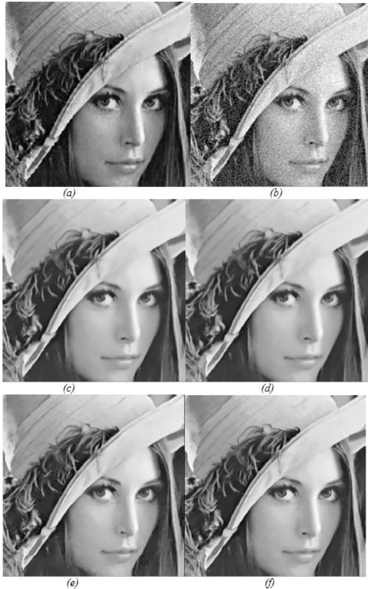
Figure 3. Lena image: (a) original image; (b) noisy image; (c)Trace based PDE method; (d) Curvature Preserving PDE method; (e) Weighted Cuvature Preserving PDE method; (f) Our method
