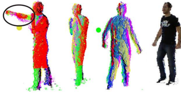
Figure 6. Image on the left shows the acquisition drift (circled) if the software synchronization is not employed. Next two images show the result of synchronous acquisition with the alignment of the dynamic point clouds. Last image shows the fusion of both RGB and depth data
