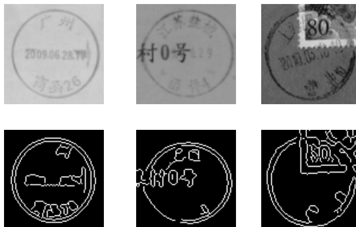
Figure 11. Postmarks and their Edges Detected by Canny Detector
