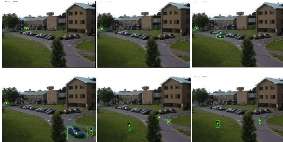
Figure 2. (b) Tracking of Multiple Moving Objects was based on 2DPCA-GMM and KF
