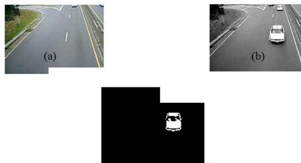
Figure 2. a) Background Image b) After Gamma Correction c) After Subtraction
