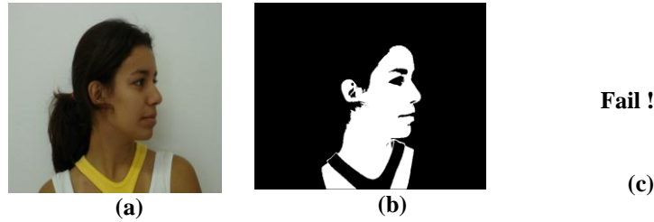
Figure 13. Clothes with Similar Skin Color Lead to Face Segmentation Error case: (a) Original Image; (b) Segmented Image; (c) Detected Face Image.
