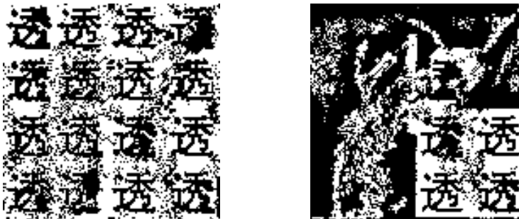
Figure 7. Watermarks extracted from watermarked JPEG2000 images compressed with file size ratios 11.8% (left) and 7.8% (right).
