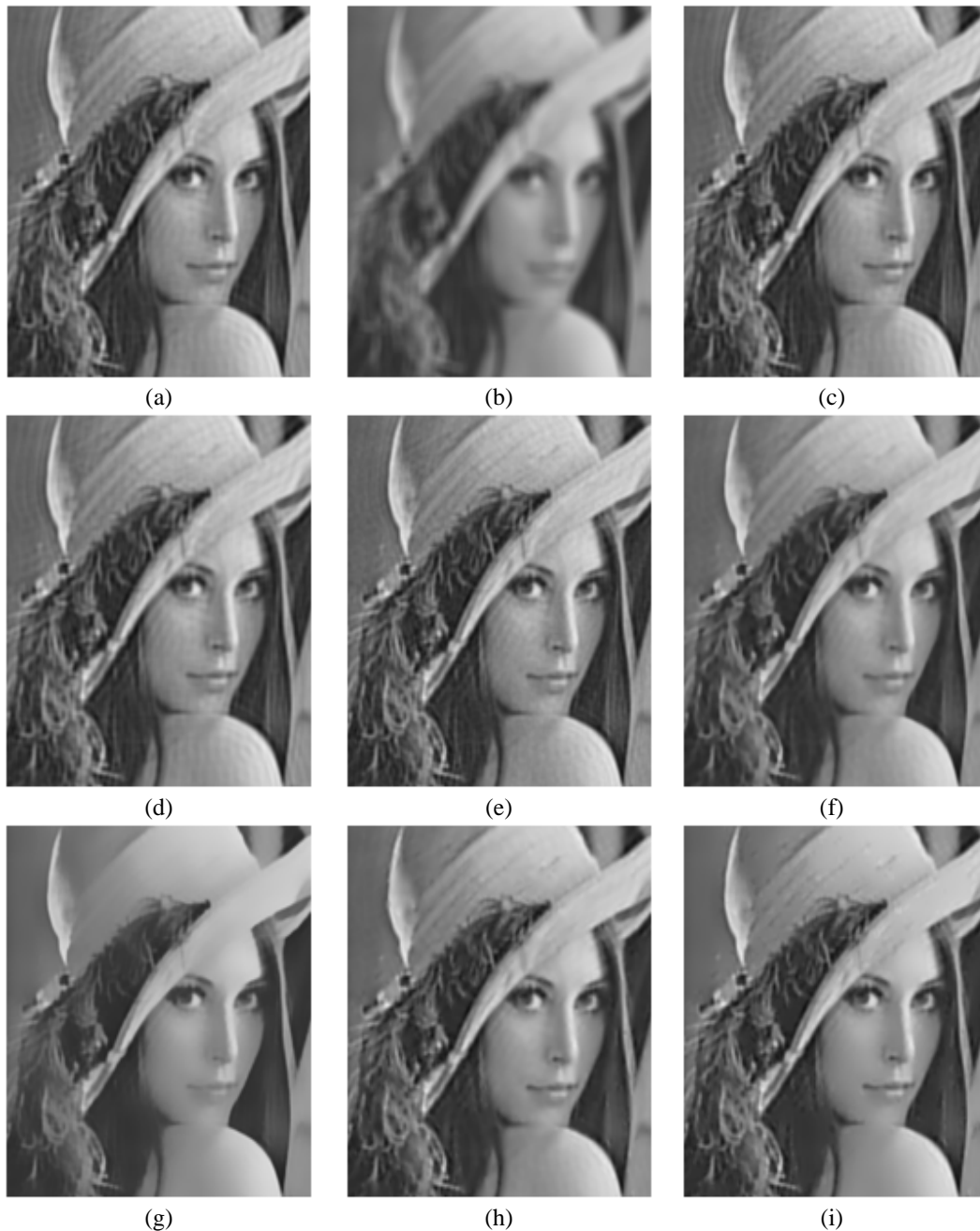
Figure. 7. (a) Original Lena image, (b) Blurred image with 11X11 uniform blur and 50dB gaussian noise, (c) Restored image by iterative method [1], (d) Restored image by adaptive iterative method, (e) Restored image by CLS filter with ringing artifact, (f) Bilateral filtering image with sigma 2, (g) Bilateral filtering image with sigma 20, (h) The result using proposed region classification and adaptive gaussian filtering (i) The result using proposed algorithm.
