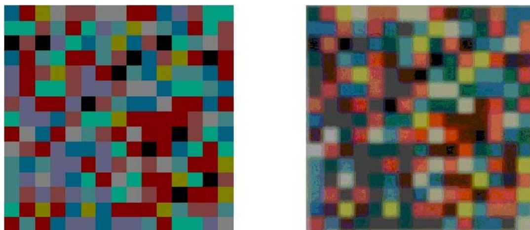
Figure 6. Comparing between a JPEG compressed 2D barcode sample image (left) and its camera phone captured equivalent (right).
