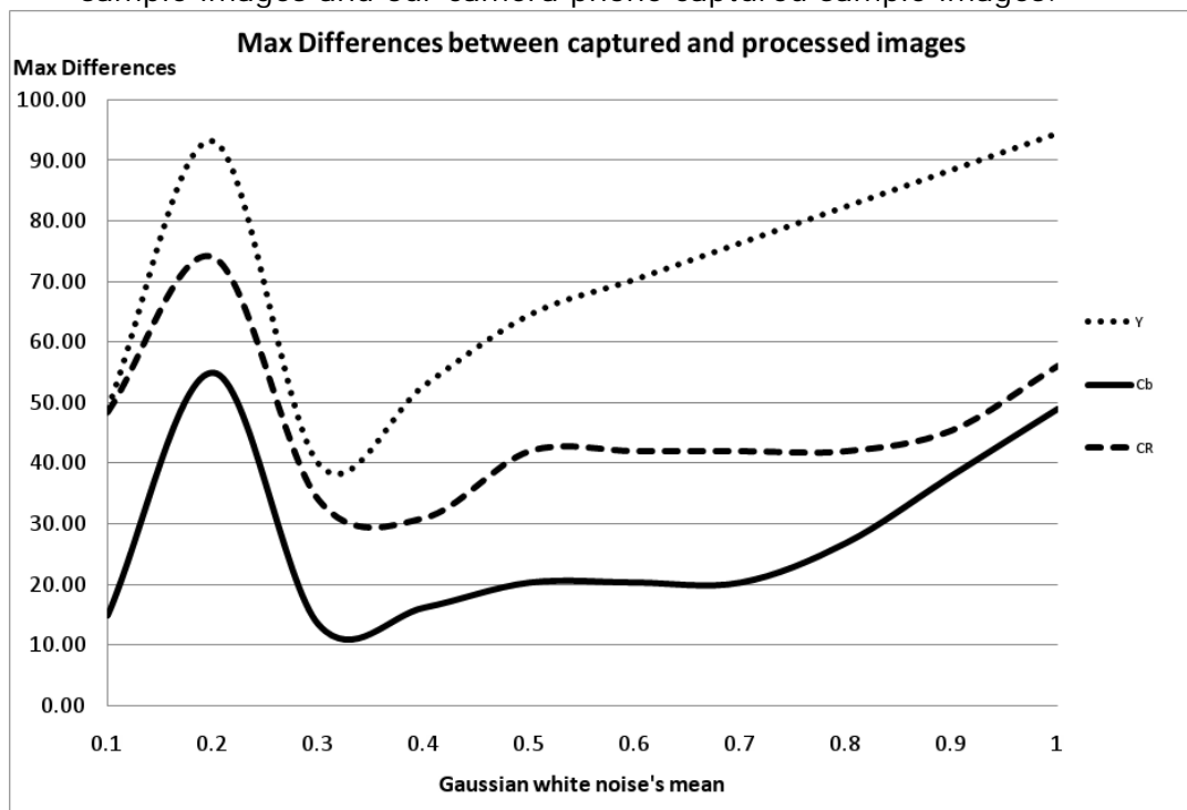
Figure 9. Maximum differences in YCbCr values between our pre-processed sample images and our camera phone captured sample images.
